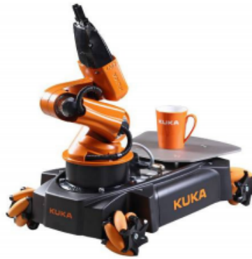
Figura 2.5: Kuka Omnidirectional Robot (Bischoff, 2011)
